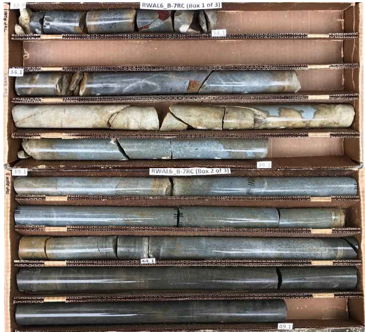
Rock Core Photographs Boring: RWAL6_B-7 32.9 to 49.1 Feet
