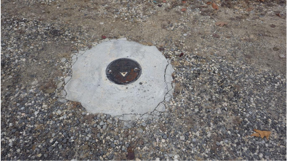
Newer monitoring well
