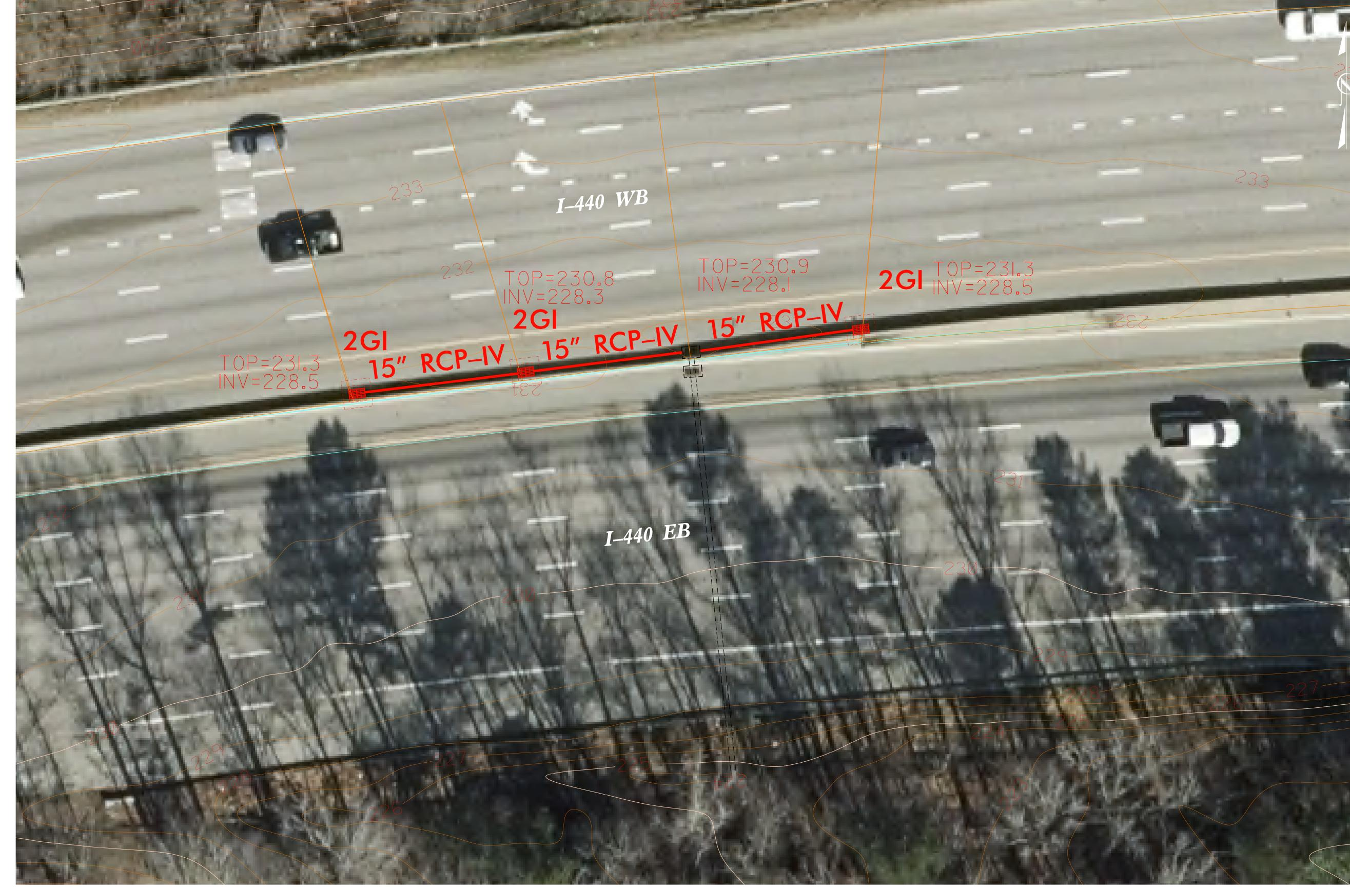
NOTE: PROPOSED PIPE EXTENSIONS AND DROP INLETS ON NORTH SIDE OF MEDIAN SHALL BE SET AT GRADES AND INVERT ELEVATIONS TO ENSURE POSITIVE FLOW TO THE EXISTING DROP INLET. INSTALLATION AT UNIFORM DEPTHS FROM THE EXISTING PAVEMENT SURFACE SHOULD PROVIDE POSITIVE FLOW. PIPE EXTENSION LAYOUT, DROP INLET LOCATIONS, AND PIPE GRADE AND INVERT ELEVATIONS SHALL BE APPROVED BY THE ENGINEER PRIOR TO INSTALLATION.
