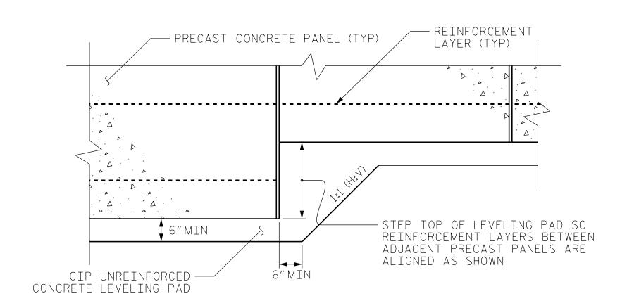
PRECAST PANELS LEVELING PAD STEP DETAIL
