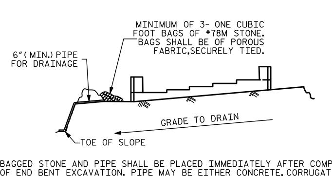
BAGGED STONE AND PIPE SHALL BE PLACED IMMEDIATELY AFTER COMPLETION OF END BENT EXCAVATION. PIPE MAY BE EITHER CONCRETE, CORRUGATED STEEL, CORRUGATED ALUMINUM ALLOY, OR CORRUGATED PLASTIC. PERFORATED PIPE WILL NOT BE ALLOWED.
