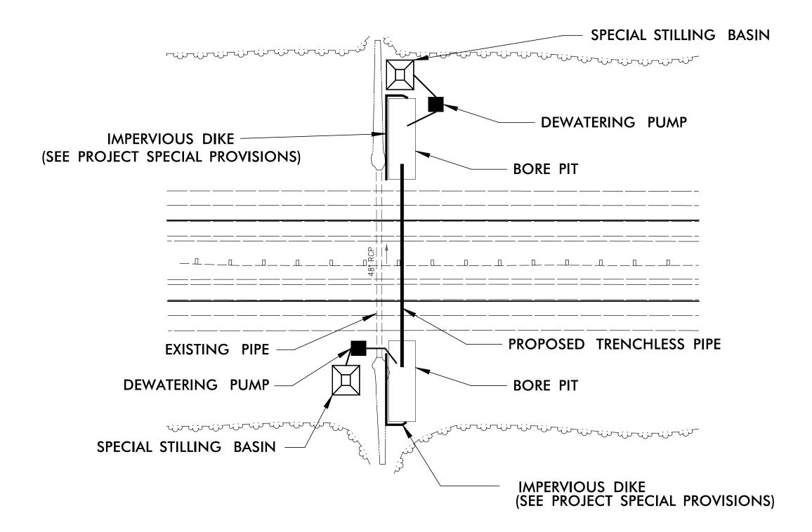
METHOD 1: CONSTRUCTION SEQUENCE FOR TYPICAL WORK AREA
