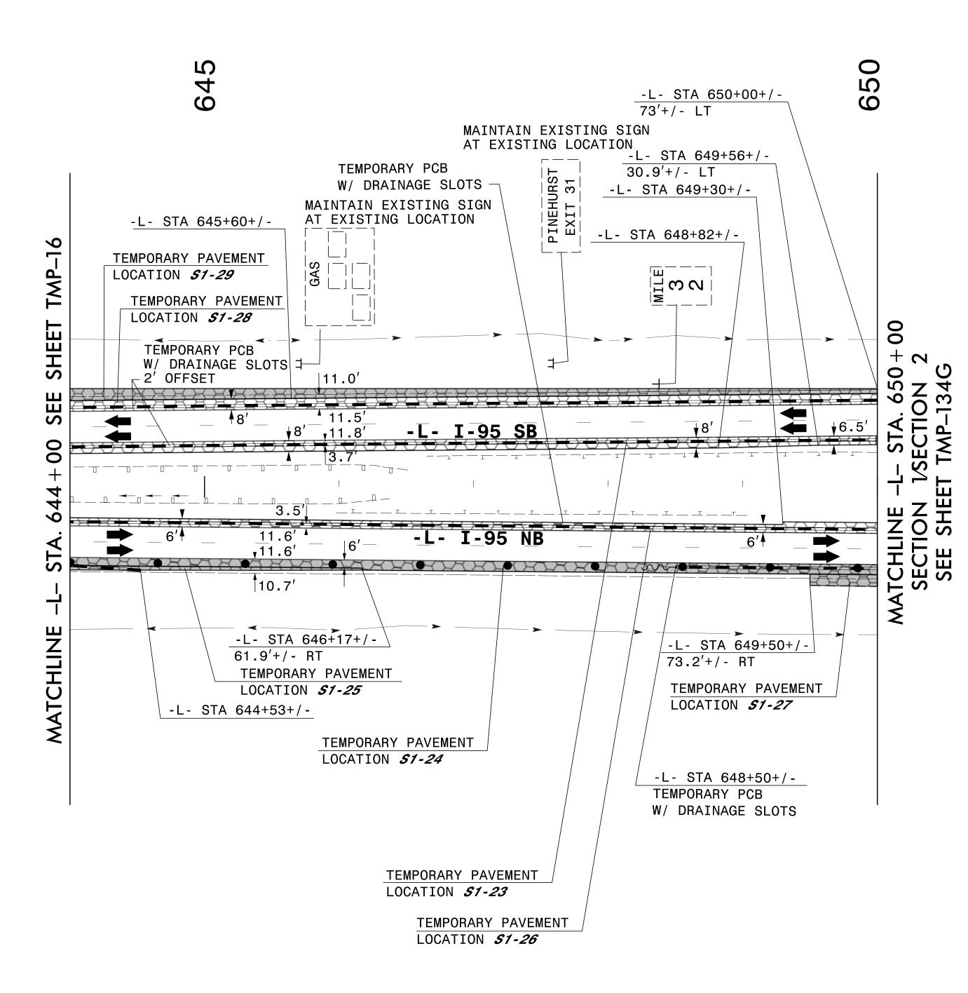
TEMPORARY PAVEMENT LOCATION *\$1-23*ON INSIDE SHOULDER OF SB I-95 ON -LFROM STA 628+36+/- TO STA 650+00+/FOR TEMPORARY TRAFFIC PATTERN
