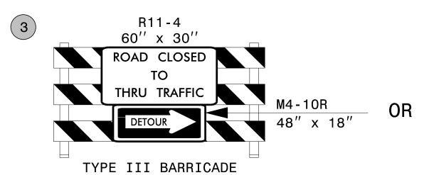
NOTE: USE "ROAD CLOSED TO THRU TRAFFIC" WHERE DISTANCE TO CLOSURE IS 1 MILE OR LESS
