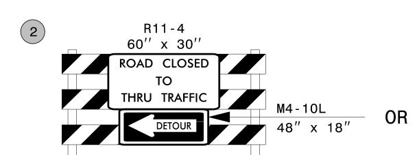
TYPE III BARRICADE NOTE: USE "ROAD CLOSED TO THRU TRAFFIC" WHERE DISTANCE TO CLOSURE IS 1 MILE OR LESS
