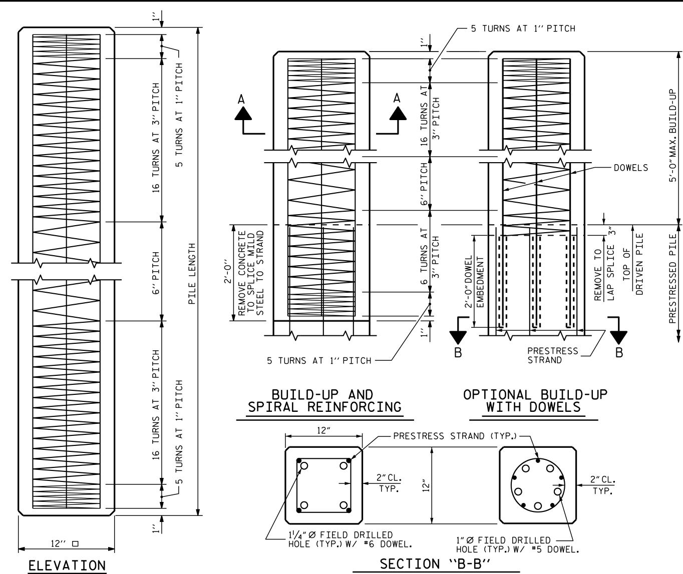
(AT THE CONTRACTOR'S OPTION, PILE BUILD-UP MAY BE CONSTRUCTED WITH DOWELS.)
