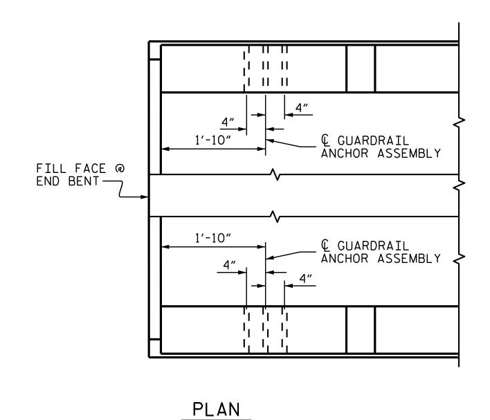
LOCATION OF GUARDRAIL ANCHOR AT END POST
