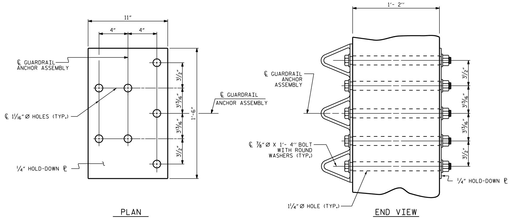
GUARDRAIL ANCHOR ASSEMBLY DETAILS
