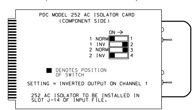
NOTE: IF ANOTHER MANUFACTURER TYPE OF AC ISOLATOR IS USED, OUTPUT PROGRAMMING IS LIKELY NOT TO EQUATE TO THAT SHOWN ABOVE.
