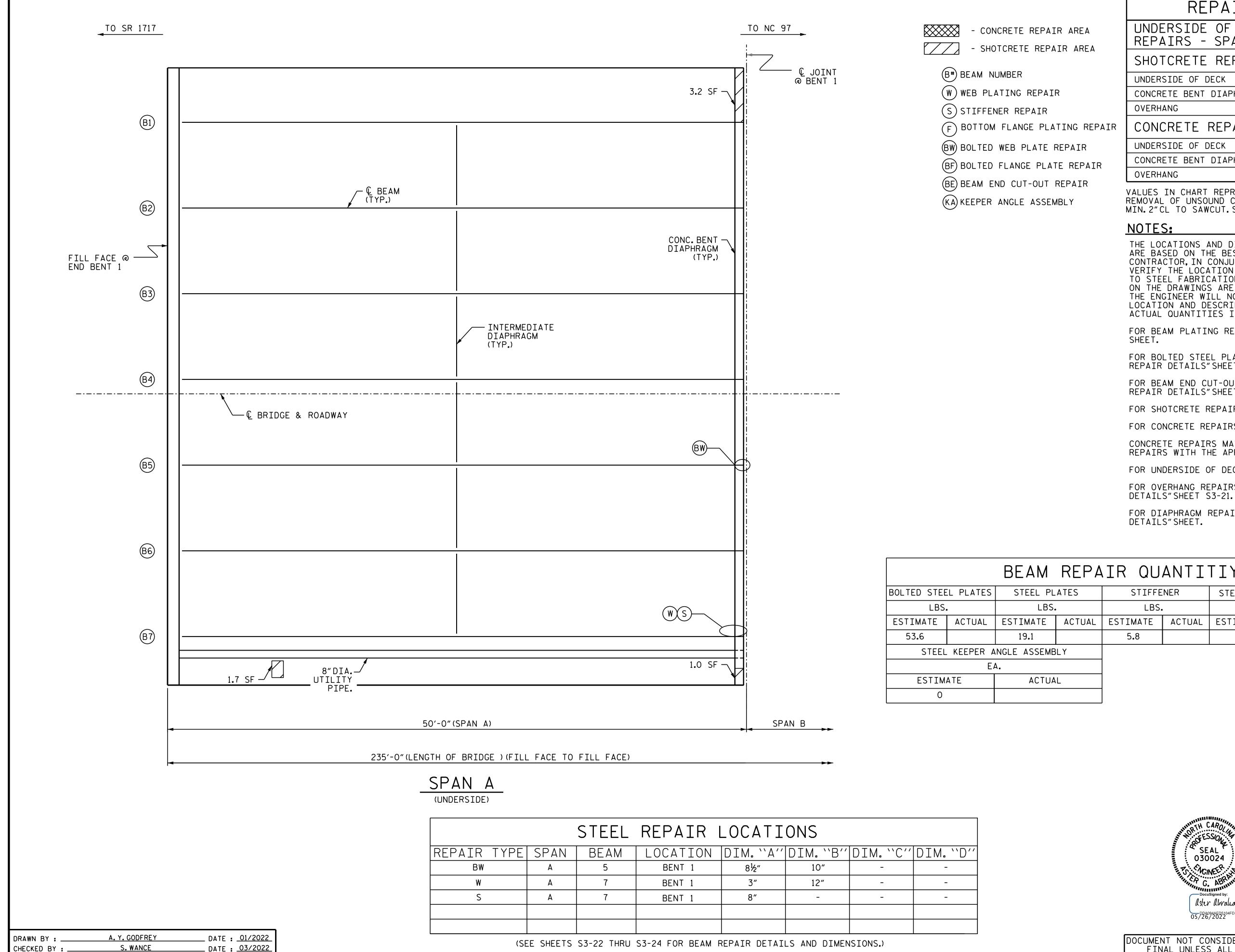
REPAIR QUANTITY TABLE UNDERSIDE OF DECK QUANTITIES REPAIRS - SPAN A ESTIMATE ACTUAL **VOLUME** AREA AREA VOLUME SHOTCRETE REPAIRS CF CF UNDERSIDE OF DECK 0.0 0.0 CONCRETE BENT DIAPHRAGM 4.2 2.1 0.6 1.7 AREA VOLUME VOLUME CONCRETE REPAIRS SF CF CF UNDERSIDE OF DECK 0.0 0.0 CONCRETE BENT DIAPHRAGM 0.0 0.0 0.0 0.0
