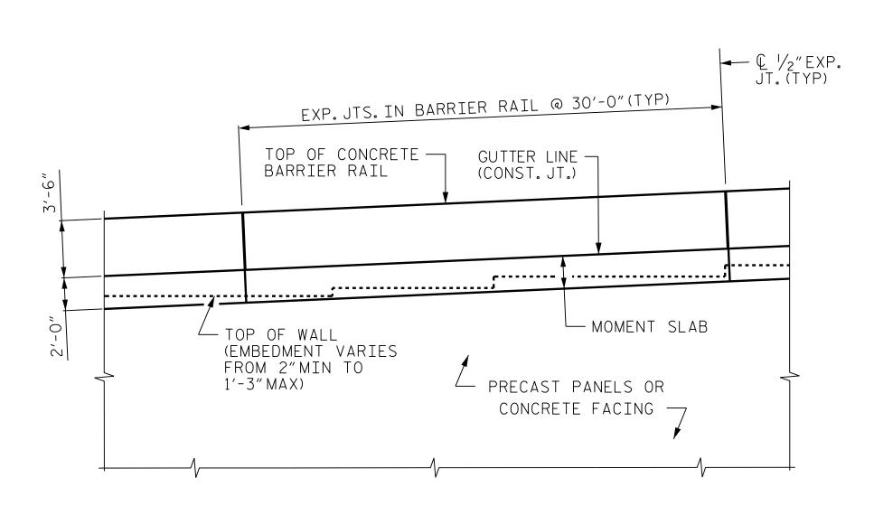
CONCRETE BARRIER RAIL WITH MOMENT SLAB - PARTIAL ELEVATION
