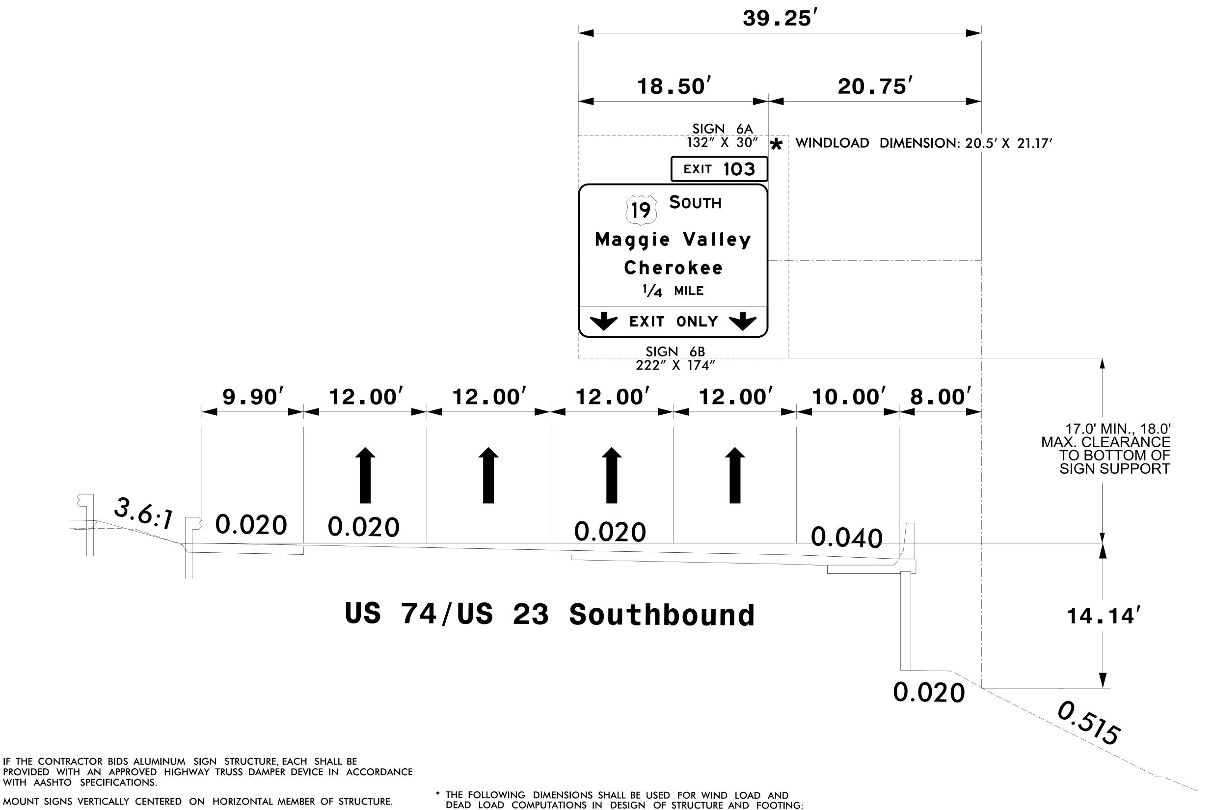
PROVIDED WITH AN APPROVED HIGHWAY TRUSS DAMPER DEVICE IN ACCORDANCE WITH AASHTO SPECIFICATIONS.
