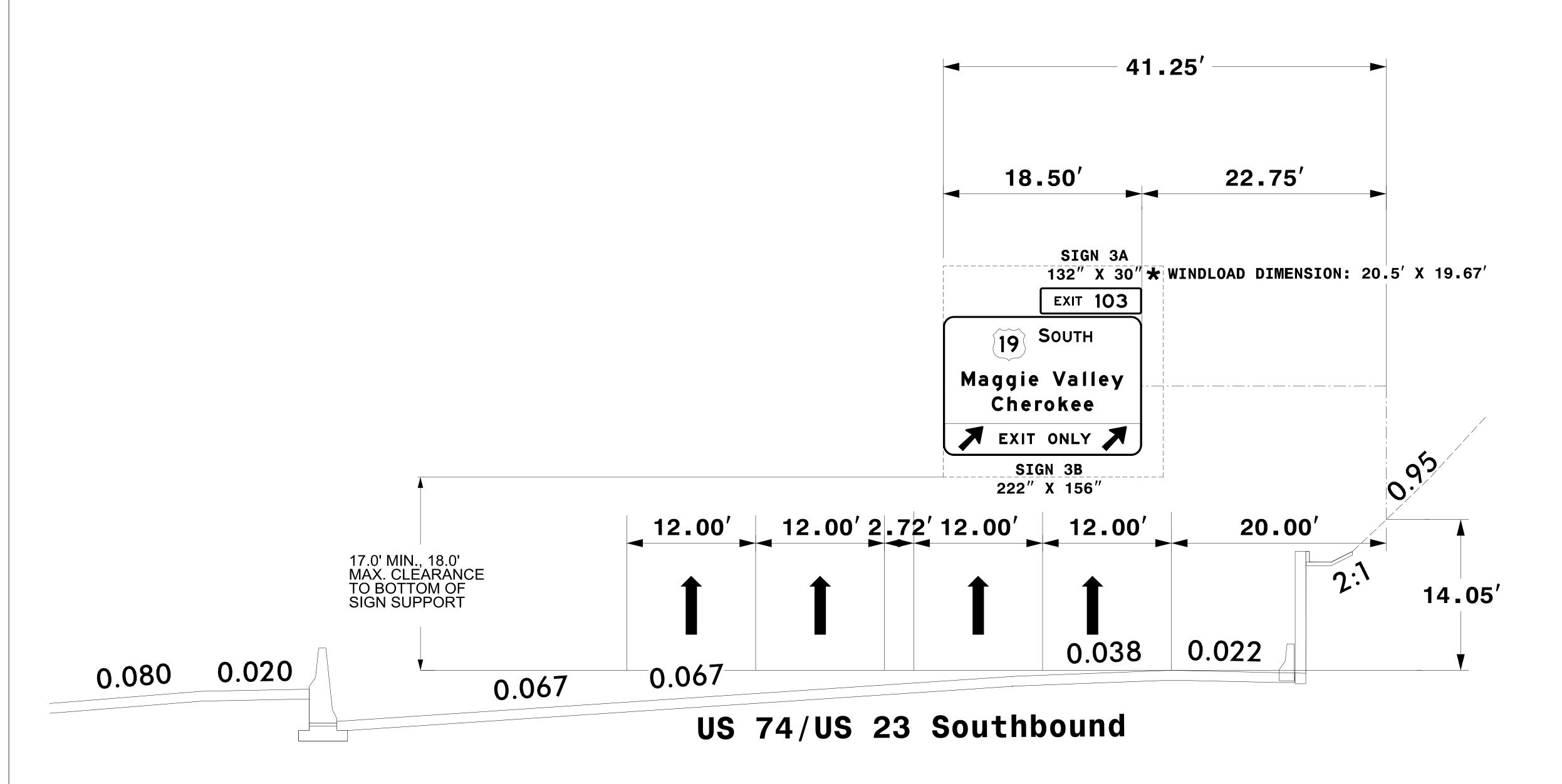
IF THE CONTRACTOR BIDS ALUMINUM SIGN STRUCTURE, EACH SHALL BE PROVIDED WITH AN APPROVED HIGHWAY TRUSS DAMPER DEVICE IN ACCORDANCE WITH AASHTO SPECIFICATIONS.
