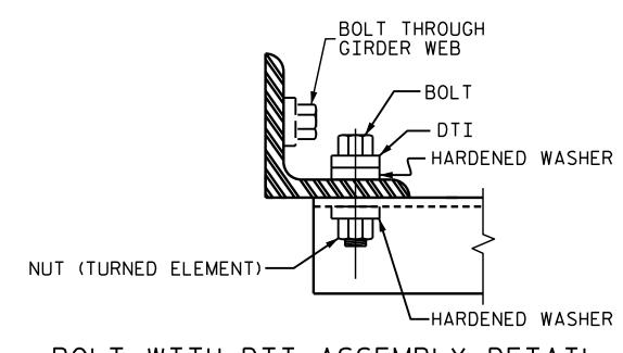
BOLT WITH DTI ASSEMBLY DETAIL
