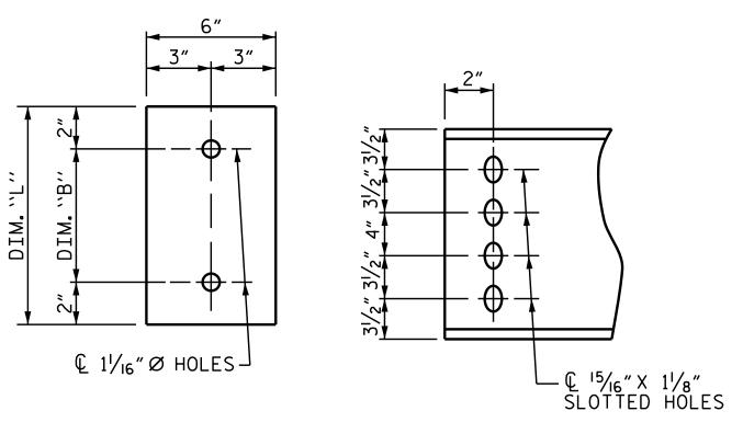
PLATE DETAILS CHANNEL END (TYPE IV GDR.)
