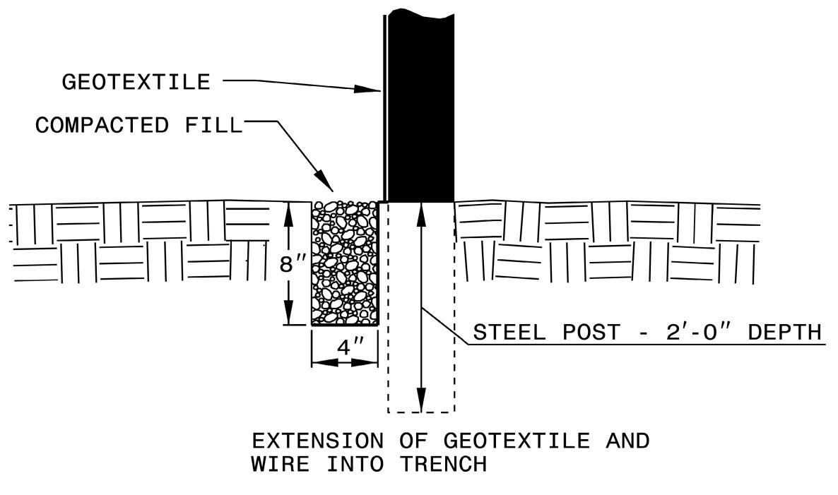
ROADWAY STANDARD DRAWING FOR TEMPORARY SILT FENCE
