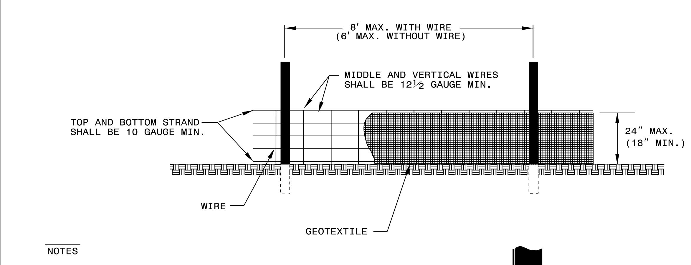
USE GEOTEXTILE A MINIMUM OF 36" IN WIDTH AND FASTEN ADEQUATELY TO THE POSTS AND WIRE AS DIRECTED.
