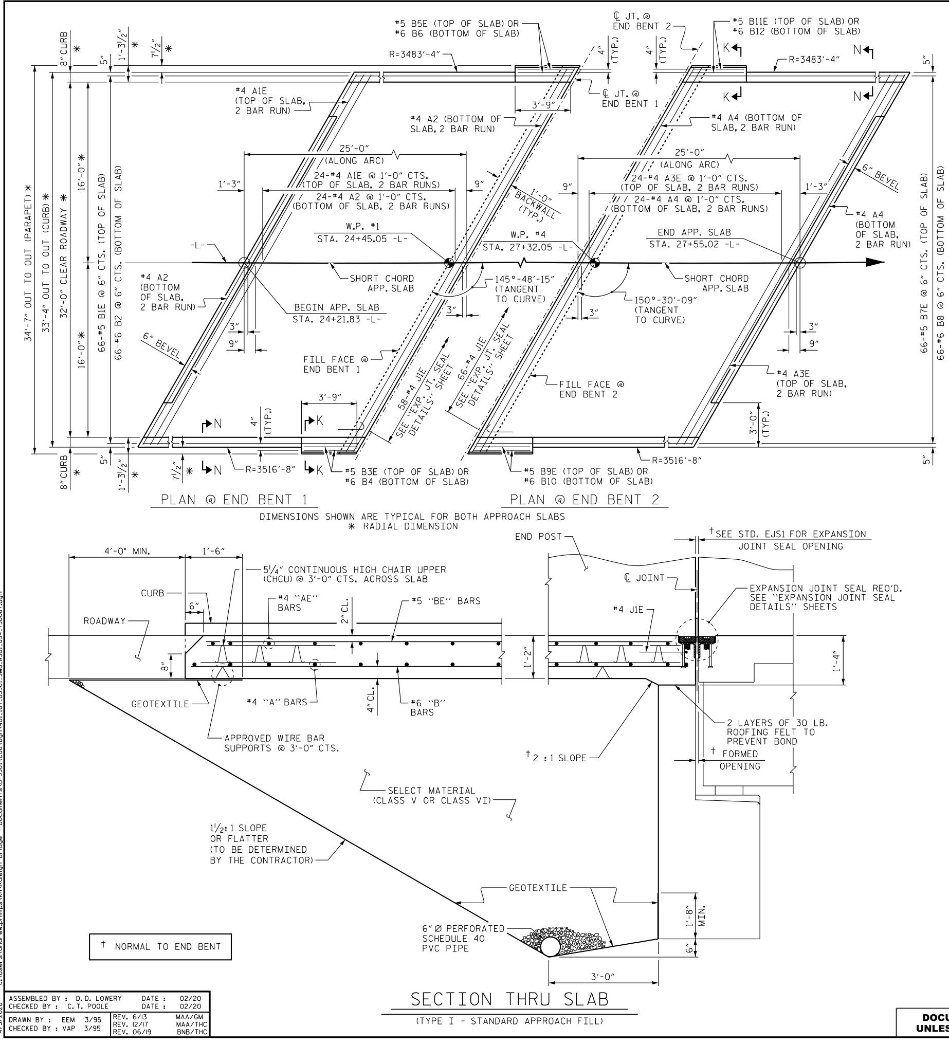
FOR BRIDGE APPROACH FILL INC AND SELECT MATERIAL BACKFILI GEOTEXTILE SHALL BE TYPE 1 I SPECIFICATIONS SECTION 1056.
