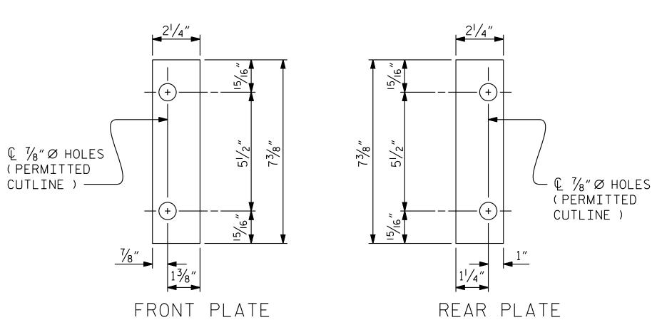
SHIM DETAILS SHIMS MAY BE CUT ALONG PERMITTED CUTLINE OR SLOTTED TO EDGE OF PLATE TO FACILITATE PLACEMENT.
