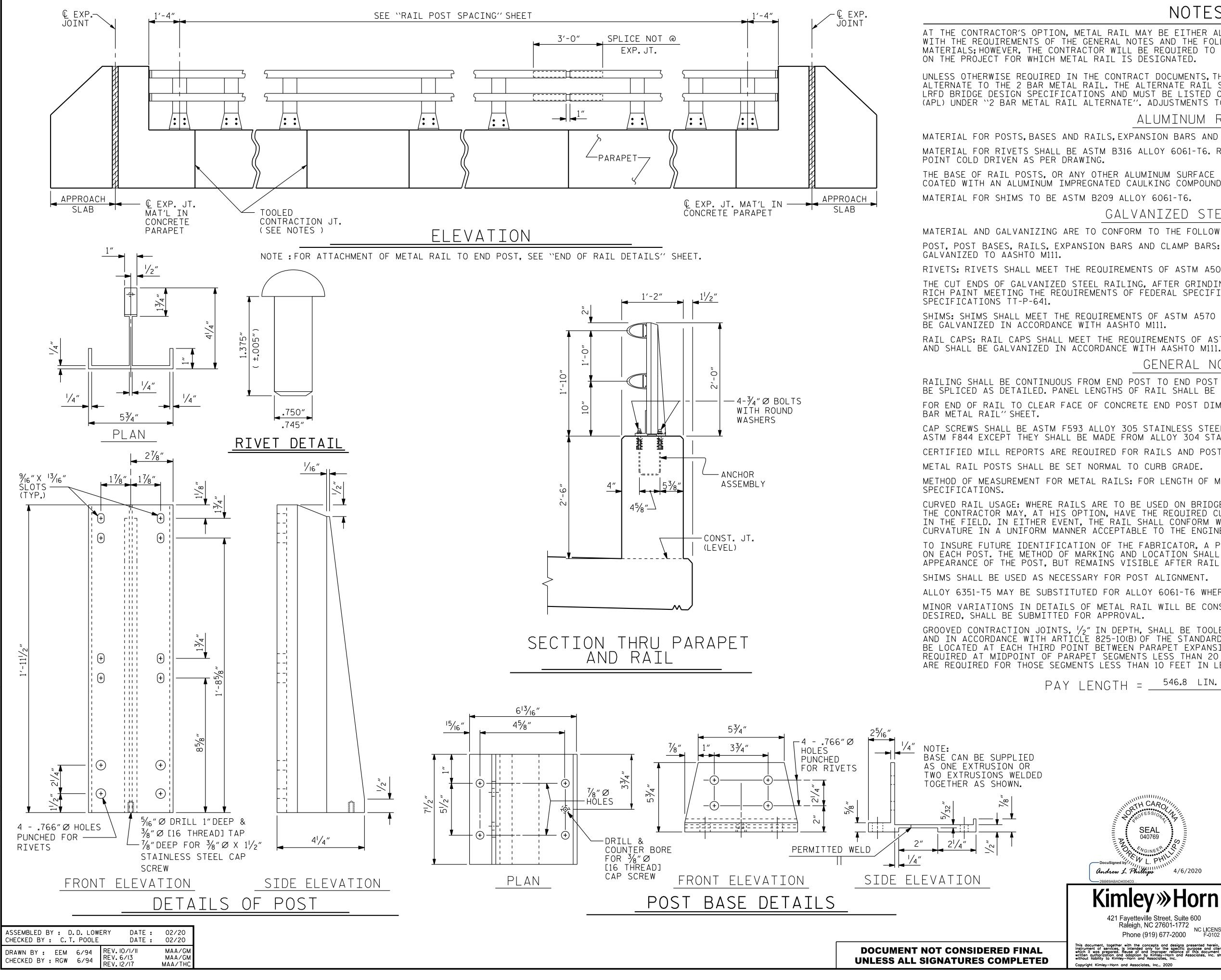
AT THE CONTRACTOR'S OPTION, METAL RAIL MAY BE EITHER ALUMINUM OR GALVANIZED STEEL IN ACCORDANCE WITH THE REQUIREMENTS OF THE GENERAL NOTES AND THE FOLLOWING SPECIFICATIONS FOR THE ALTERNATE MATERIALS; HOWEVER, THE CONTRACTOR WILL BE REQUIRED TO USE THE SAME RAIL MATERIAL ON ALL STRUCTURES ON THE PROJECT FOR WHICH METAL RAIL IS DESIGNATED.
