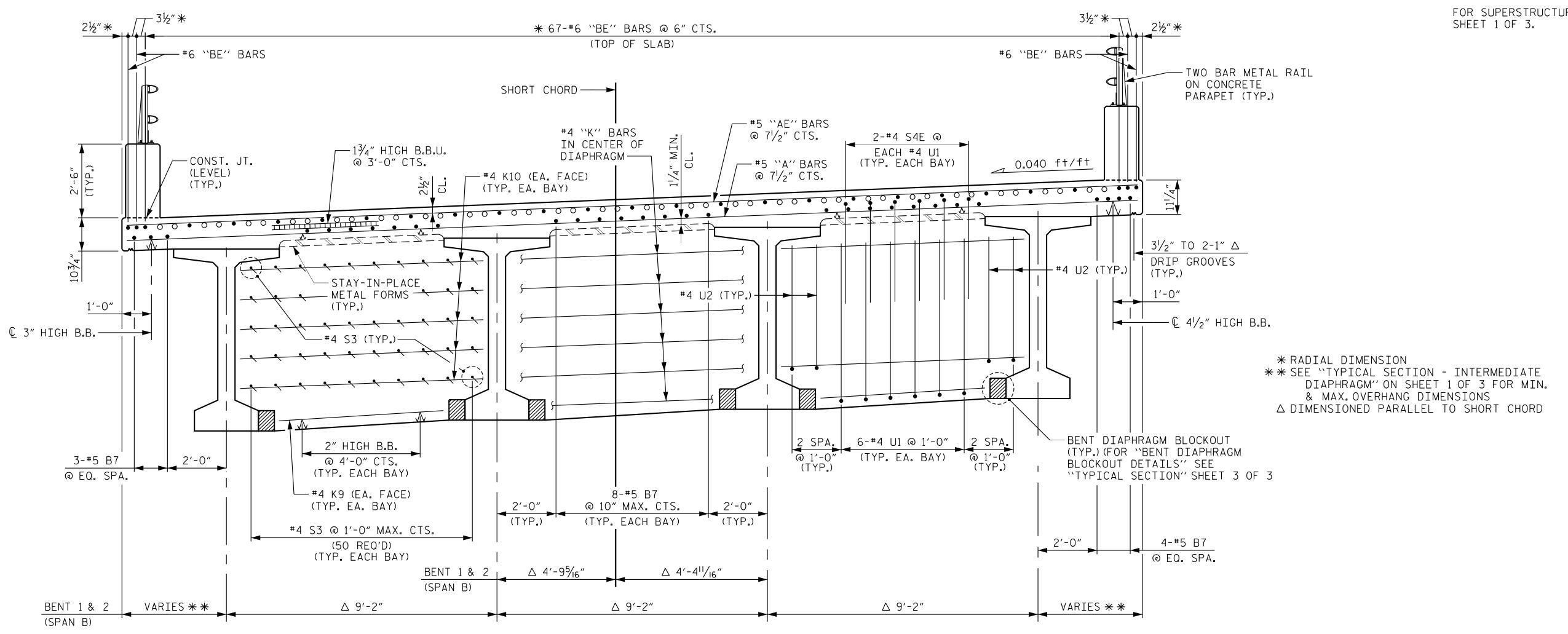
TYPICAL SECTION - BENT DIAPHRAGM
