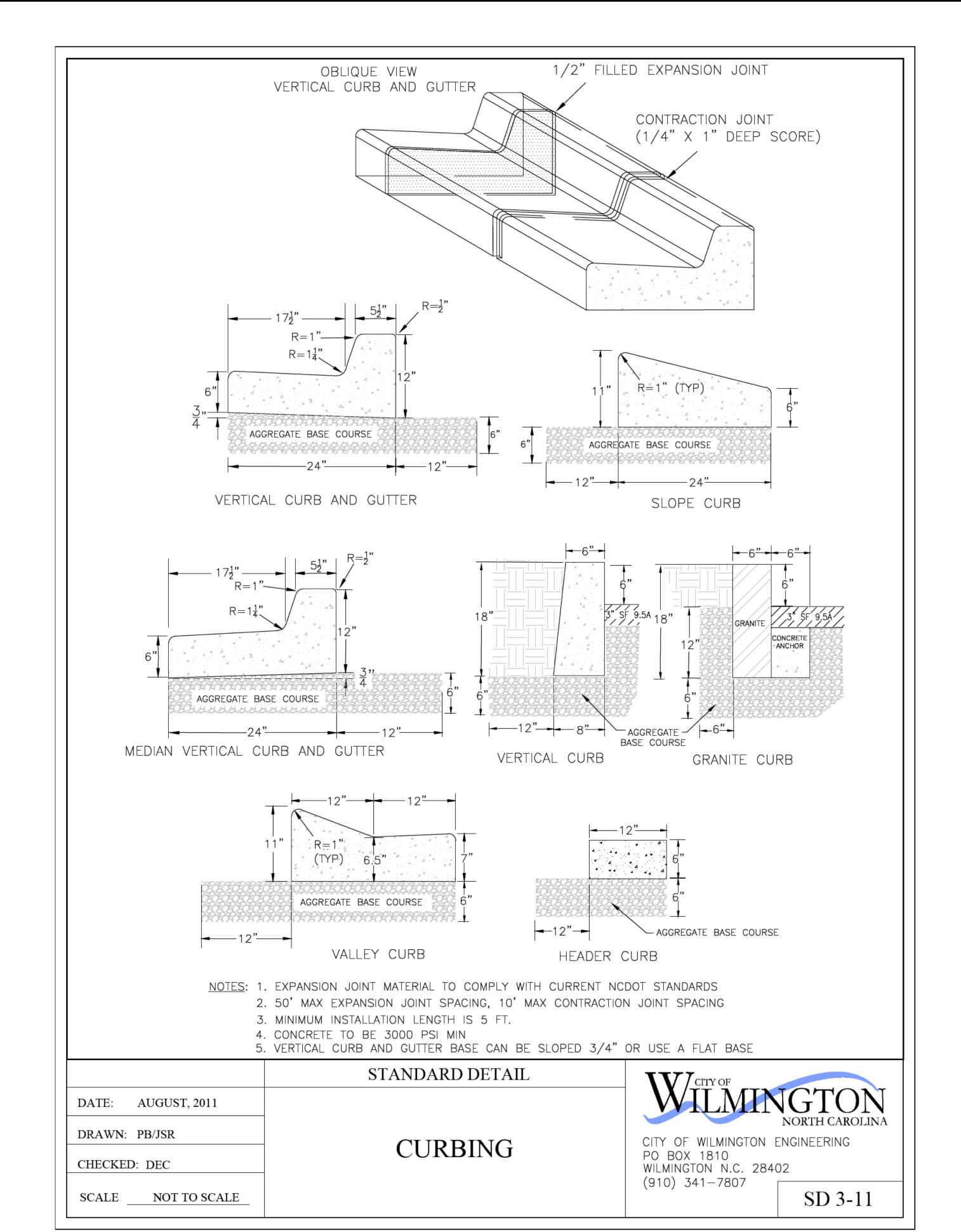
NOTE: ONLY USE VALLEY CURB DIMENSIONS FOR PLACEMENT OF SPECIAL VALLEY GUTTER. ALL OTHER CURBS SHALL BE PLACED BY NCDOT STD. 846.01.
