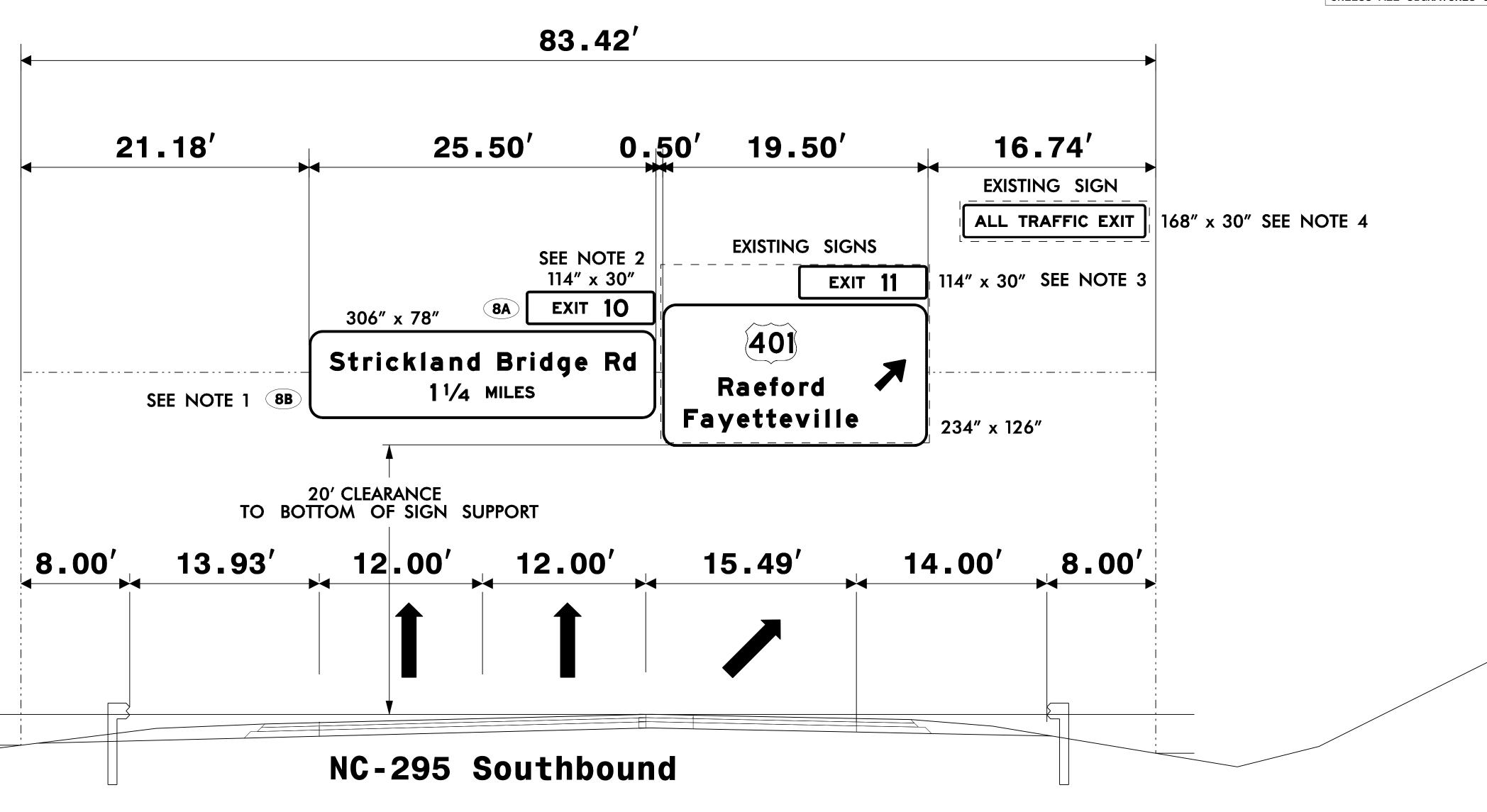
EXISTING OVERHEAD SIGN ASSEMBLY "BB" -L- STA 640 + 50
