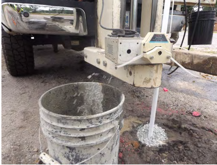
Photograph 12. Purging the temporary well prior to groundwater sample collection.
