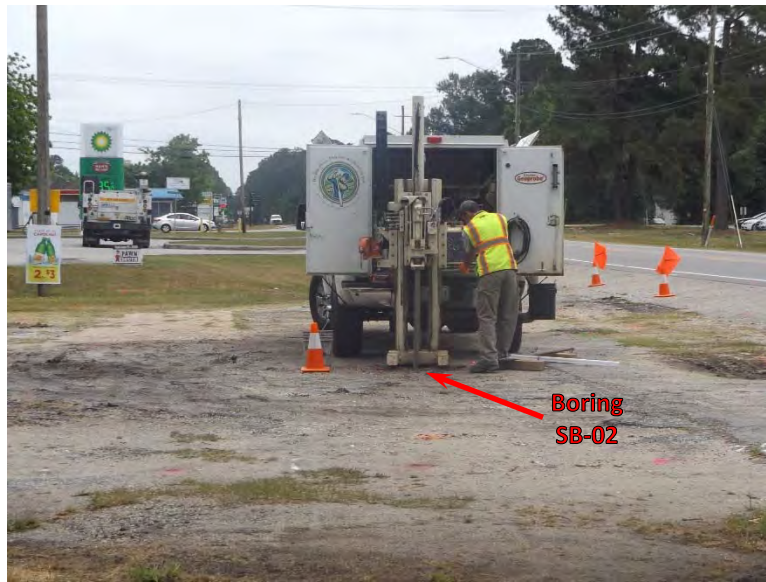
Photograph 8. GeoEnvironmental soil boring SB-R5819-02.
