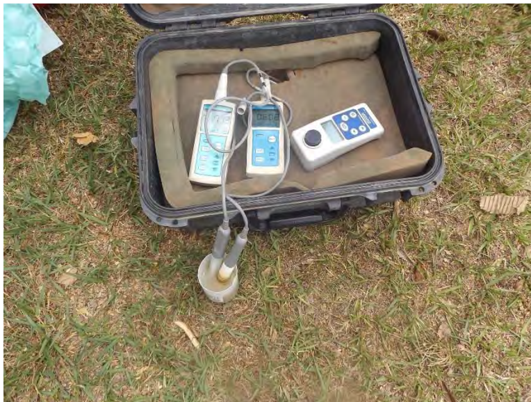
Photograph 13. Groundwater sample field parameter measurements.
