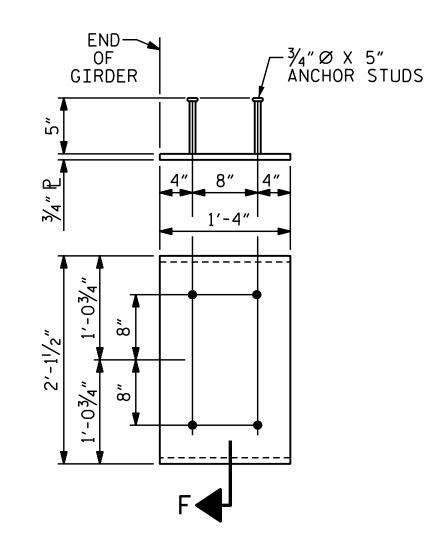
EMBEDDED PLATE "B-1" DETAILS FOR AASHTO TYPE IV GIRDER AND 63" MODIFIED BULB TEES
