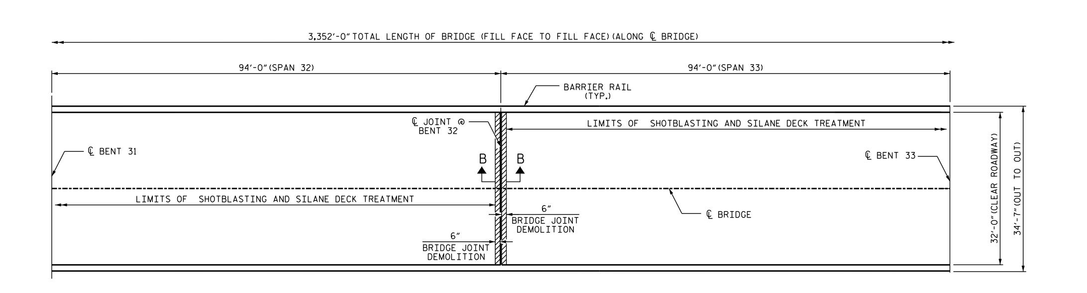
3,352'-0" TOTAL LENGTH OF BRIDGE (FILL FACE TO FILL FACE) (ALONG ← BRIDGE) 94'-0"(SPAN 34) 94'-0"(SPAN 35) BARRIER RAIL (TYP.) € JOINT @ BENT 34 LIMITS OF SHOTBLASTING AND SILANE DECK TREATMENT LIMITS OF SHOTBLASTING AND SILANE DECK TREATMENT — Ç BRIDGE € BENT 35-BRIDGE JOINT DEMOLITION € BENT 33 ---BRIDGE JOINT DEMOLITION
