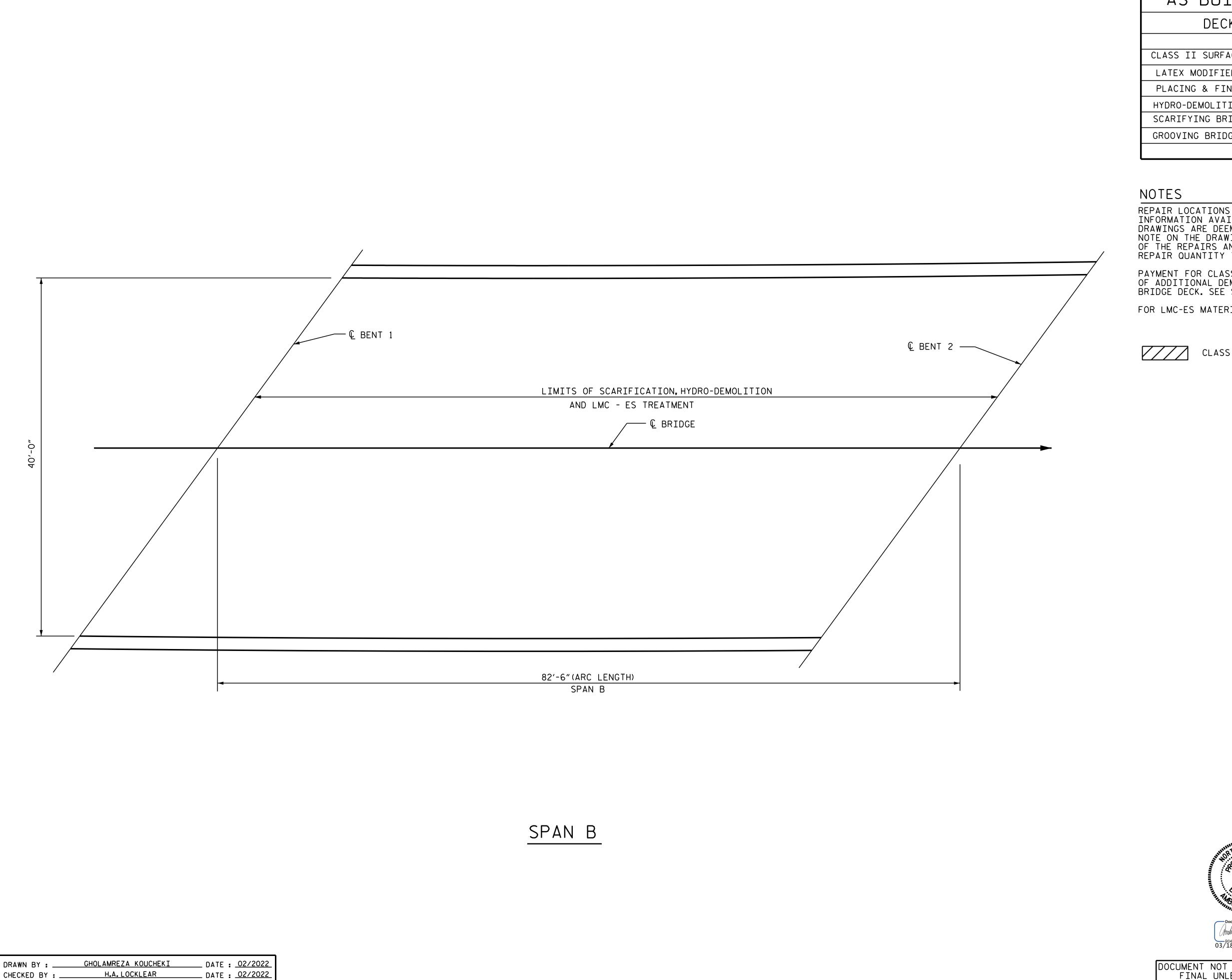
AS-BUILT REPAIR QUANTITY TABLE DECK SURFACE REPAIR - SPAN B ESTIMATE ACTUAL CLASS II SURFACE PREPARATION 0.0 SQ. YDS. 22.9 CU. YDS. LATEX MODIFIED CONCRETE-ES PLACING & FINISHING LMC-ES OVERLAY 367.0 SQ. YDS. HYDRO-DEMOLITION OF BRIDGE DECK 367.0 SQ. YDS. SCARIFYING BRIDGE DECK 367.0 SQ. YDS. 3052.0 SQ.FT. GROOVING BRIDGE FLOORS
