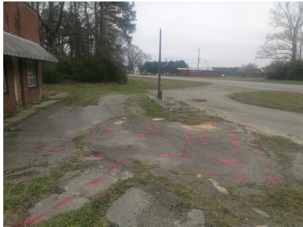
D. Photo of marked location of probable USTs, looking south
