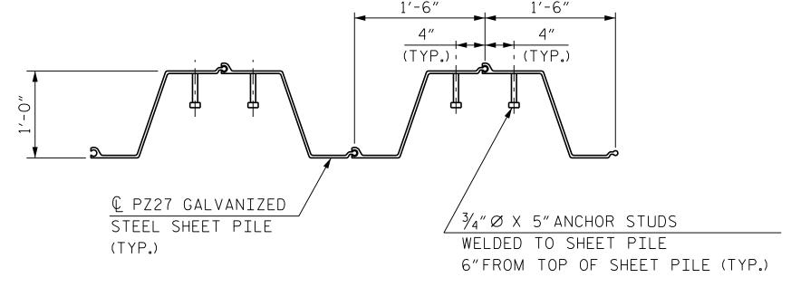
SHEET PILE ANCHOR STUD DETAILS
