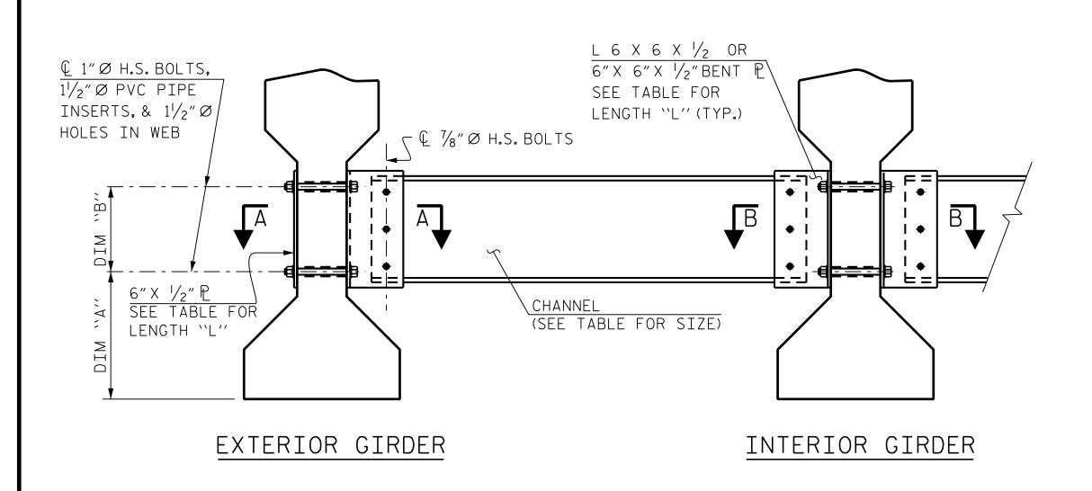
PART SECTION AT INTERMEDIATE DIAPHRAGM
