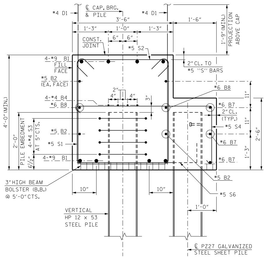
(DIMENSIONS SHOWN ARE NORMAL TO THE END BENT)
