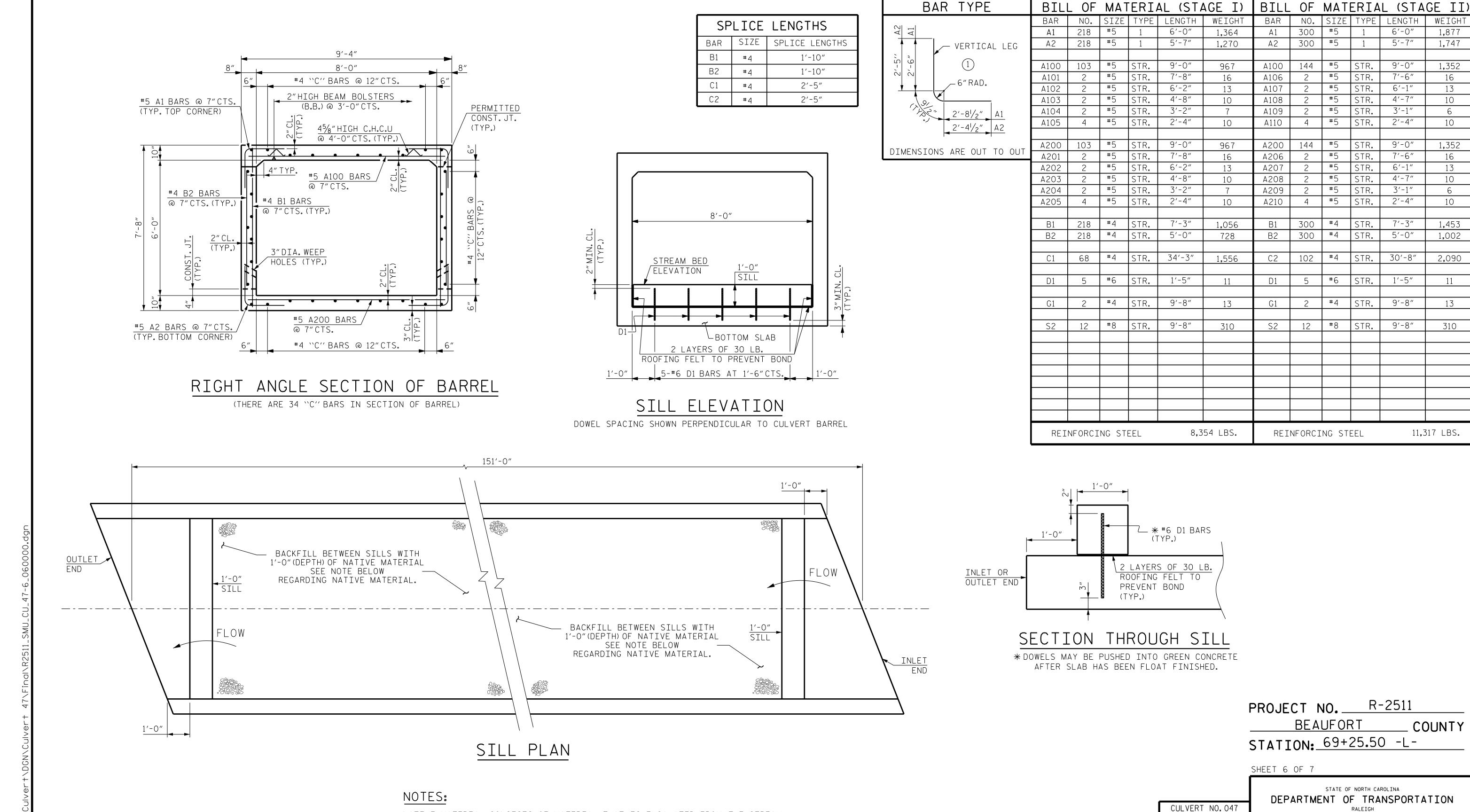
NATIVE MATERIAL CONSISTS OF MATERIAL THAT IS EXCAVATED FROM THE STREAM BED OR FLOODPLAIN AT THE PROJECT SITE DURING CULVERT CONSTRUCTION. ONLY MATERIAL THAT IS EXCAVATED FROM THE STREAMBED MAY BE USED TO LINE THE BOTTOM OF THE CULVERT BARREL.
