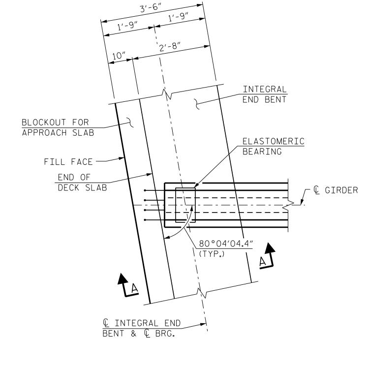
PLAN OF GIRDER AT INTEGRAL END BENT
