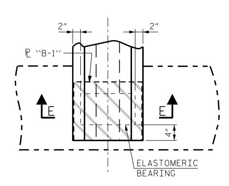
TYPICAL PLAN (INTEGRAL END BENT)
