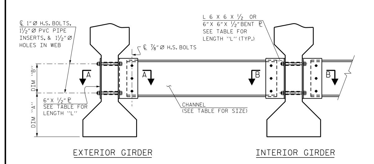
PART SECTION AT INTERMEDIATE DIAPHRAGM
