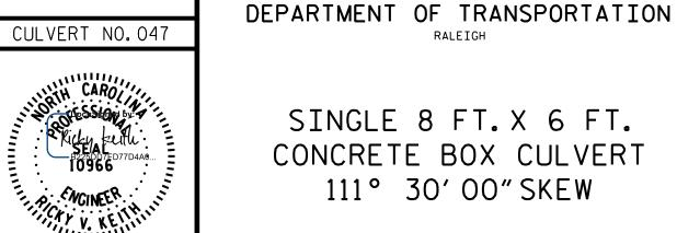
SINGLE 8 FT. X 6 FT. CONCRETE BOX CULVERT 111° 30′ 00″ SKEW
