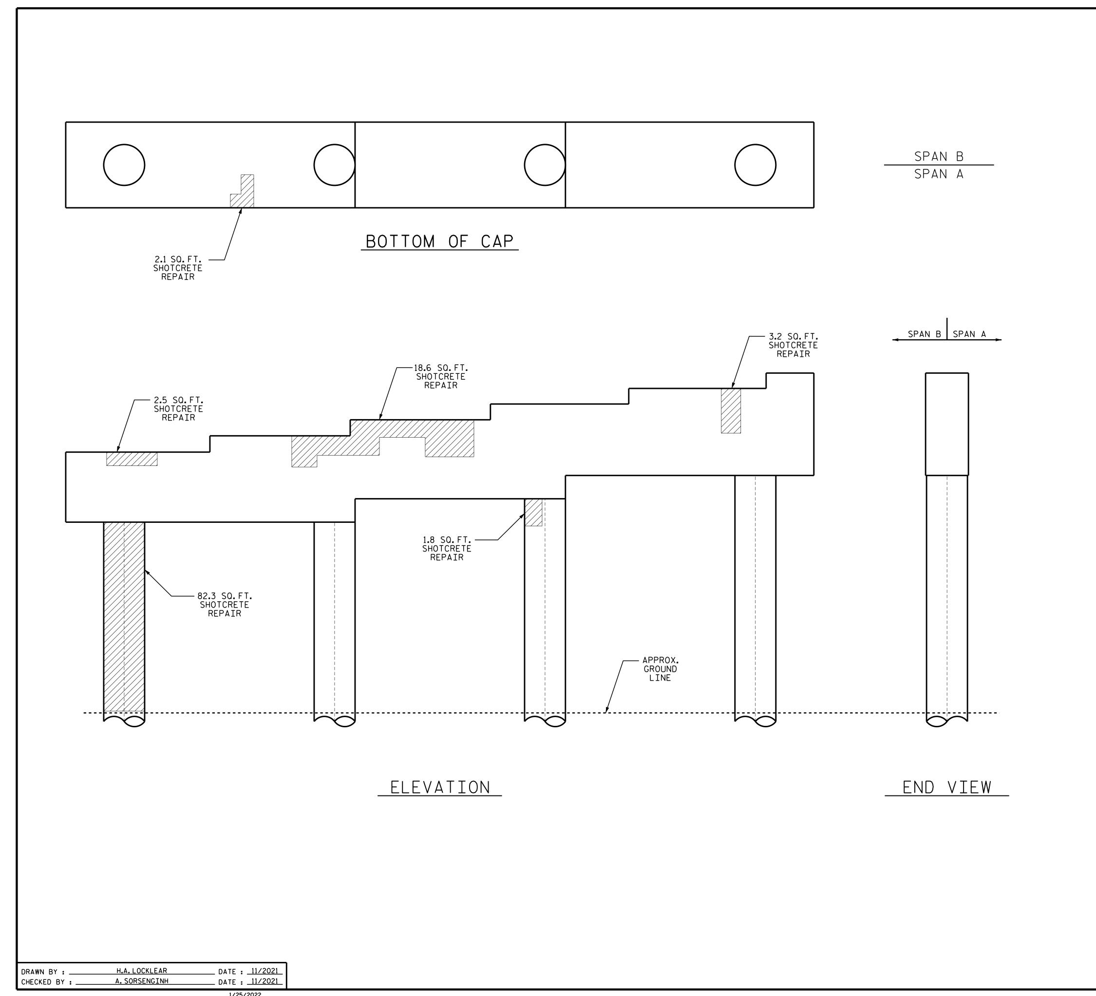
AS-BUILT REPAIR QUANTITY TABLE QUANTITIES BENT 1 SPAN B FACE ESTIMATE ACTUAL AREA SQ.FT. VOLUME CU.FT. VOLUME SHOTCRETE REPAIRS SQ.FT. CU.FT. CAP 13.2 26.4 COLUMNS 42.1 84.1 AREA SQ.FT. VOLUME **VOLUME** CONCRETE REPAIRS CU.FT. SQ.FT. CU.FT. 0.0 0.0 CAP EPOXY RESIN INJECTION LIN.FT LIN.FT CAP 0.0 0.0 COLUMNS
