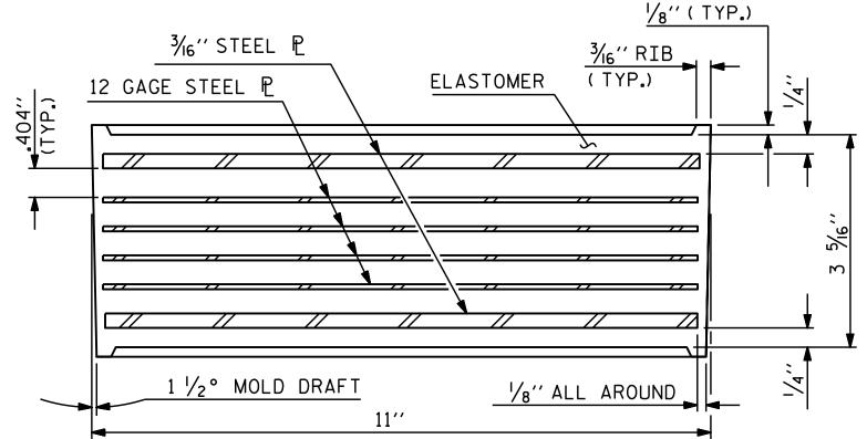
TYPICAL SECTION OF ELASTOMERIC BEARING
