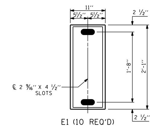
PLAN VIEW OF ELASTOMERIC BEARING
