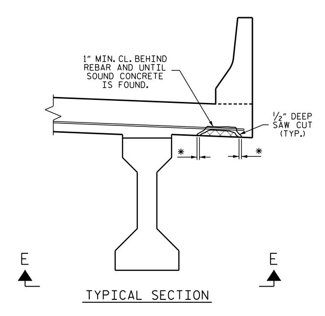
\* REMOVE CONCRETE UNTIL SOUND CONCRETE IS FOUND (2" MIN.CL.)
