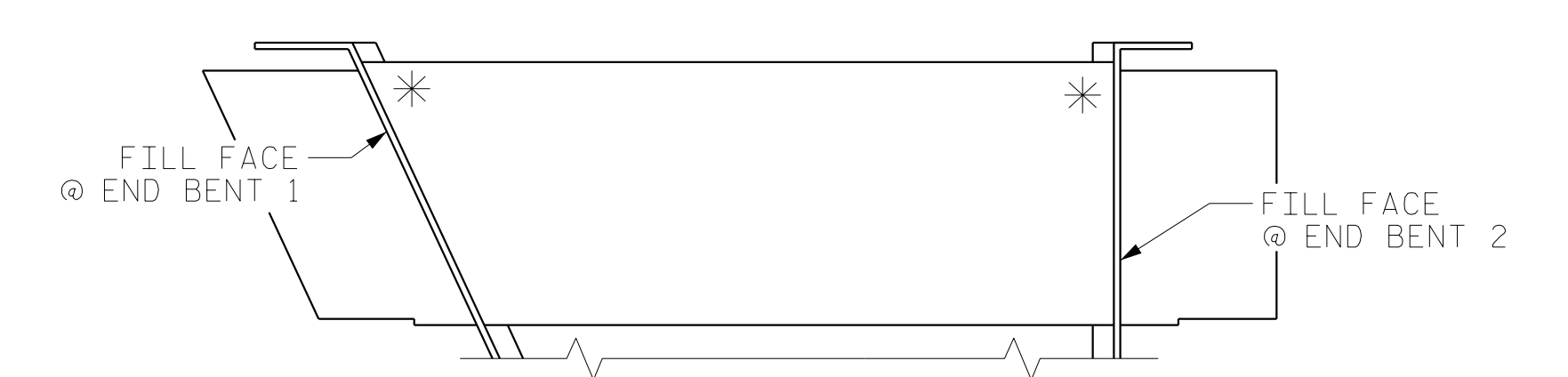
SKETCH SHOWING POINTS OF ATTACHMENT * DENOTES LOCATION OF GUARDRAIL ATTACHMENT
