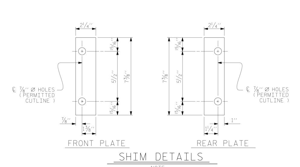
NOTE : SHIMS MAY BE CUT ALONG PERMITTED CUTLINE OR SLOTTED TO EDGE OF PLATE TO FACILITATE PLACEMENT.
