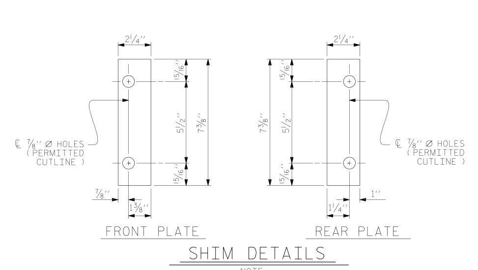
NOTE : SHIMS MAY BE CUT ALONG PERMITTED CUTLINE OR SLOTTED TO EDGE OF PLATE TO FACILITATE PLACEMENT.
