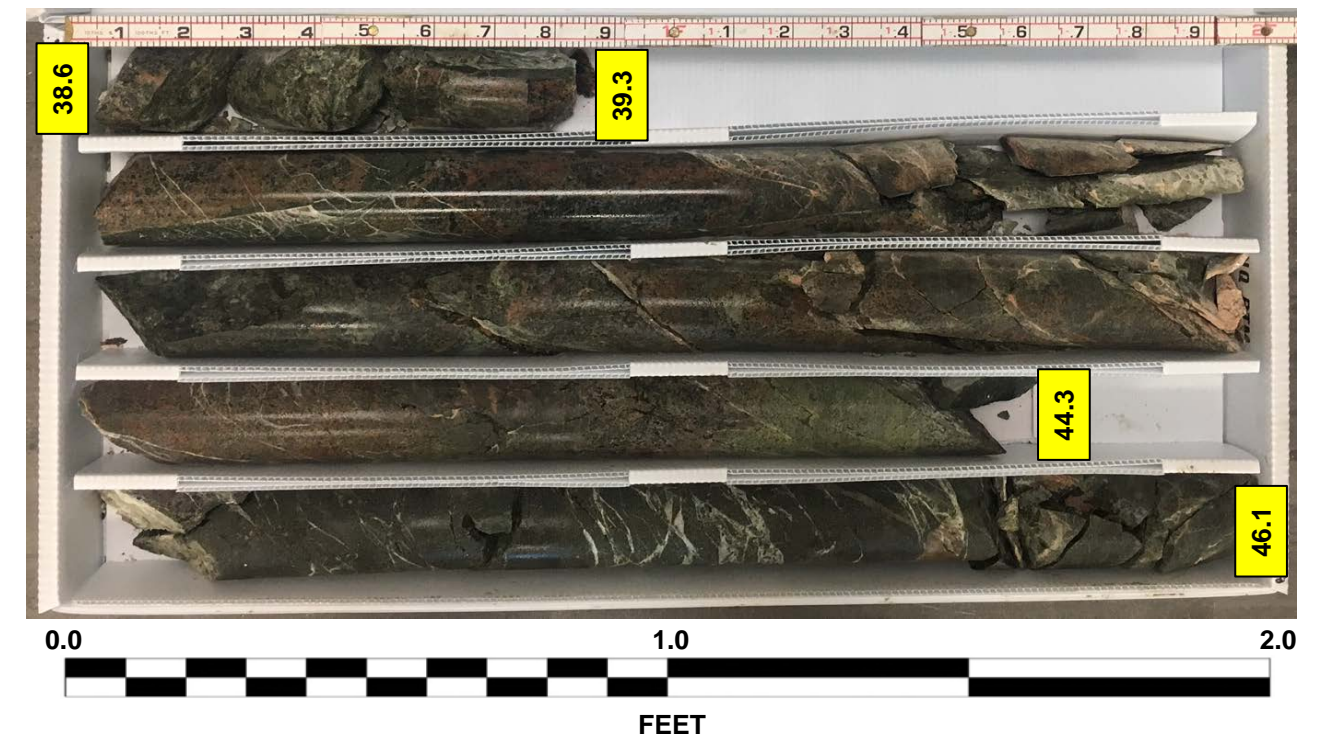
U-5738 – EB1-C STA. 27+53 @ 27' Rt. Box 2 of 4: 7.5 FEET WET
