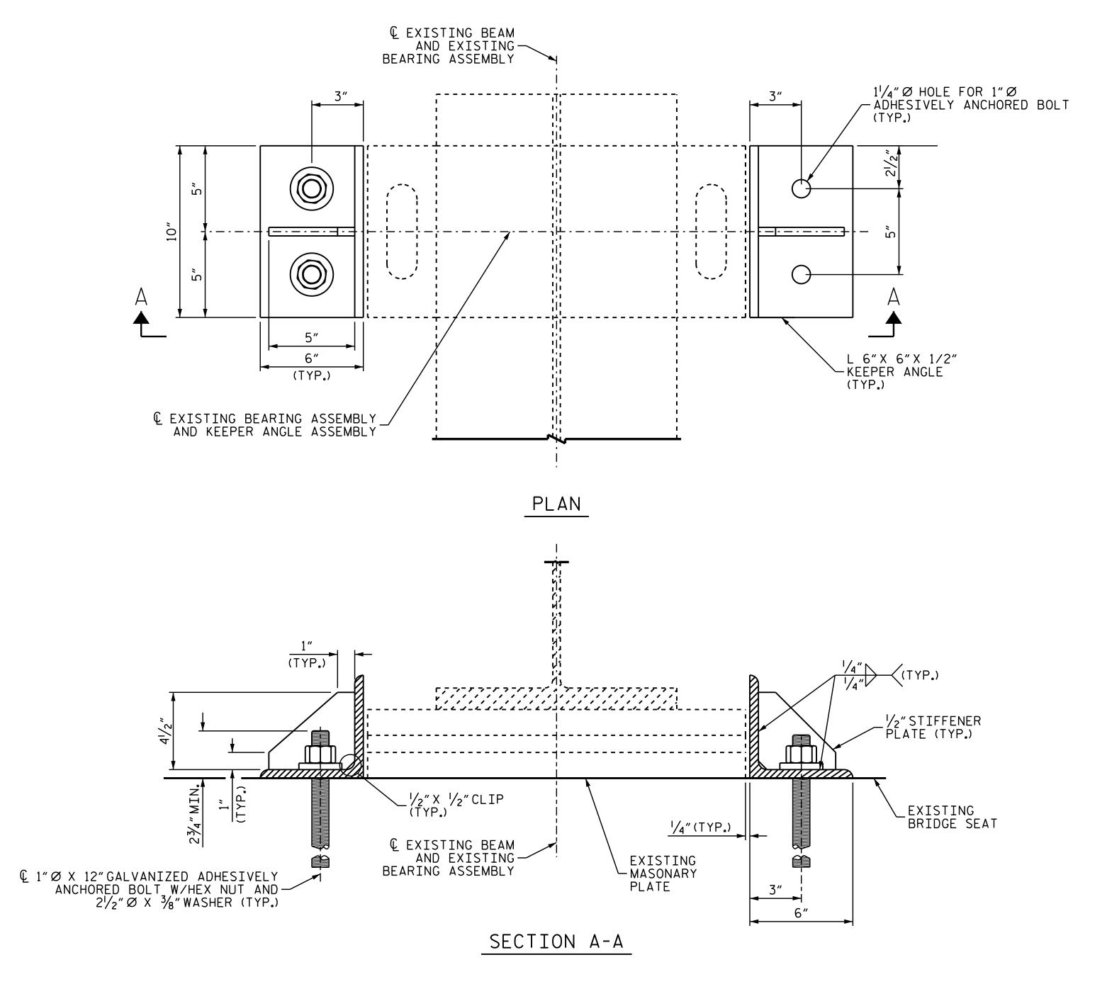
STEEL KEEPER ANGLE ASSEMBLY DETAILS
