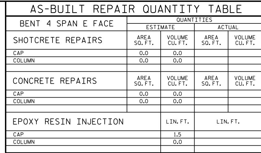
VALUES IN CHART REPRESENT ESTIMATED REPAIR TOTALS AFTER REMOVAL OF UNSOUND CONCRETE, MINIMUM OF 1"BEHIND REBAR AND MINIMUM 2"CLEARANCE TO SAWCUT. SEE "TYPICAL CAP AND COLUMN REPAIR DETAILS" SHEET.
