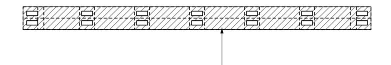
COAT ALL THE FREE SURFACE AREA ON THE TOP OF THE CAPS, INCLUDING CHAMFERS, WITH EPOXY PROTECTIVE COATING. DO NOT COAT UNDER BEARING
