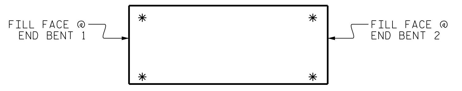
SKETCH SHOWING POINTS OF ATTACHMENTS * DENOTES GUARDRAIL ANCHOR ASSEMBLY
