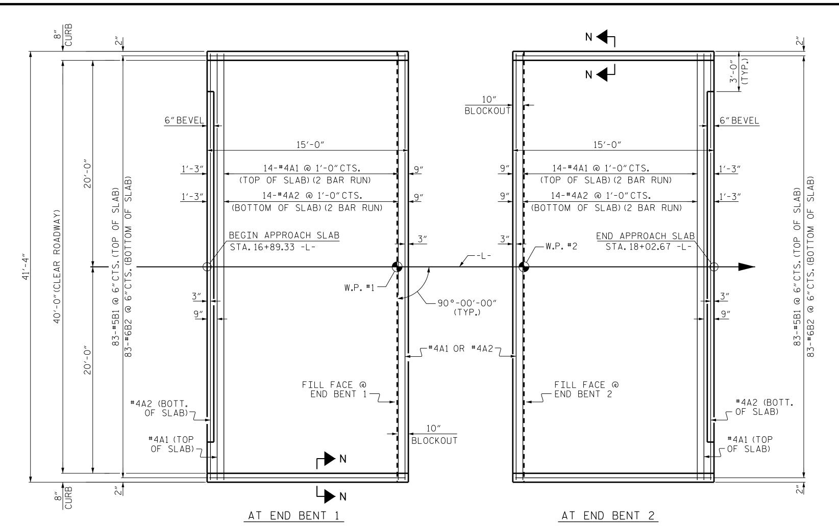
DIMENSIONS SHOWN ARE TYPICAL FOR BOTH APPROACH SLABS
