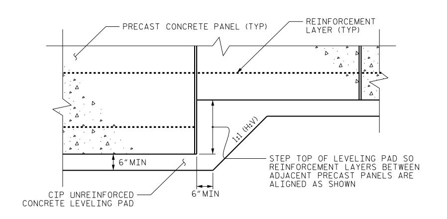
PRECAST PANELS LEVELING PAD STEP DETAIL
