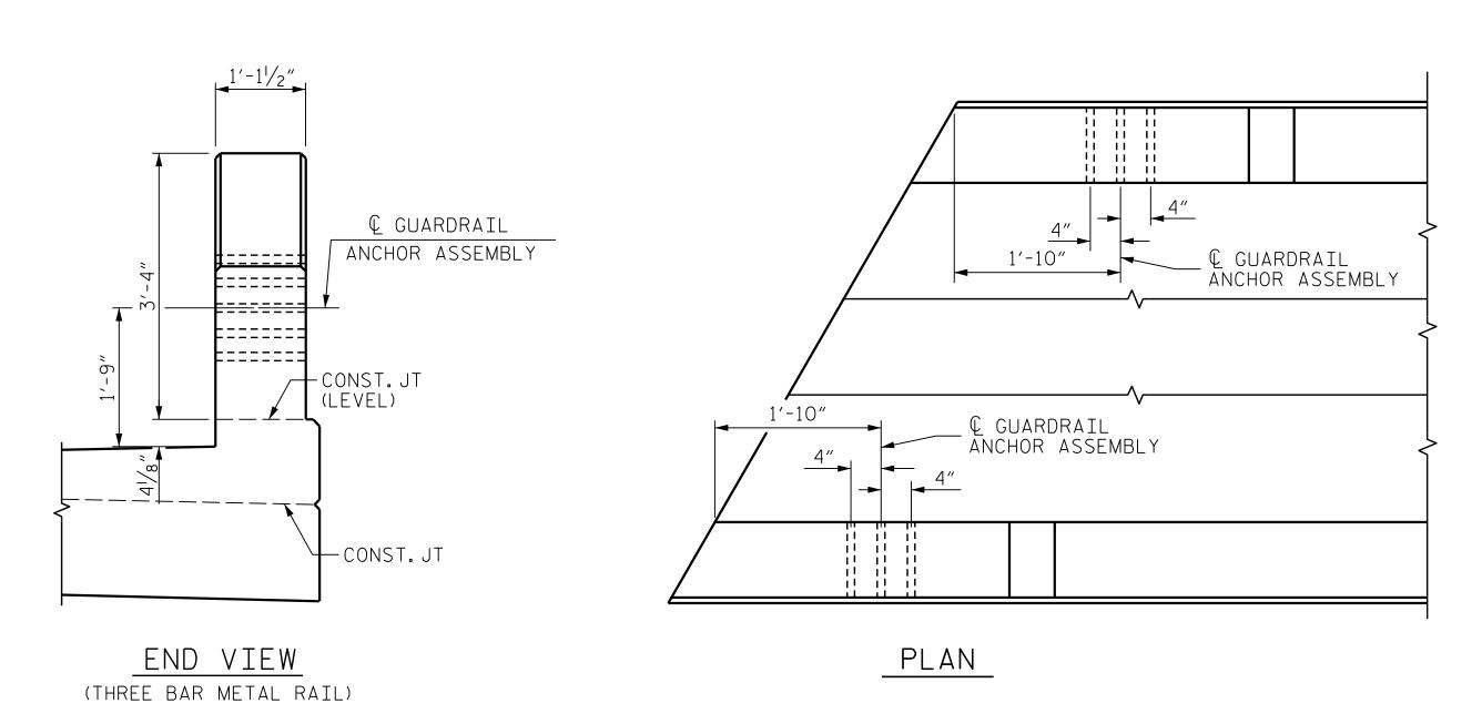
LOCATION OF GUARDRAIL ANCHOR AT END POST
