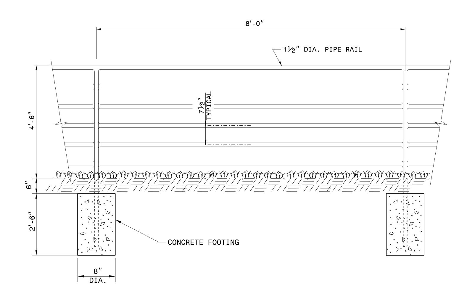
**ELEVATION OF HANDRAIL**
