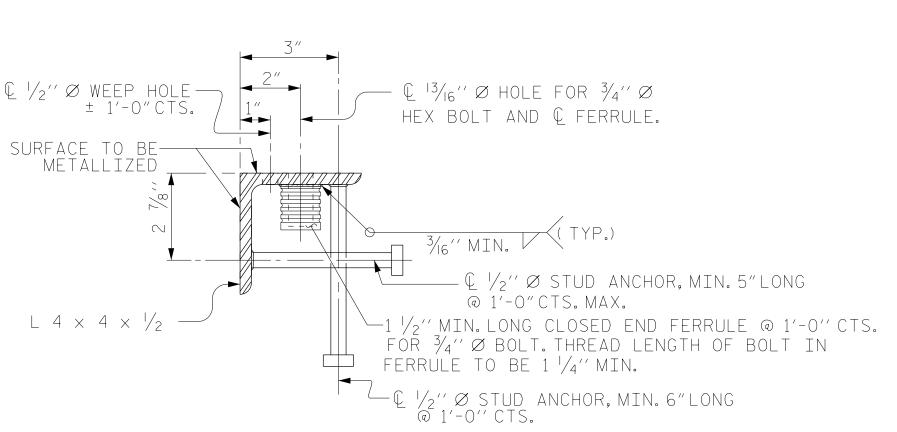
TYPICAL SECTION OF BASE ANGLE ASSEMBLY
