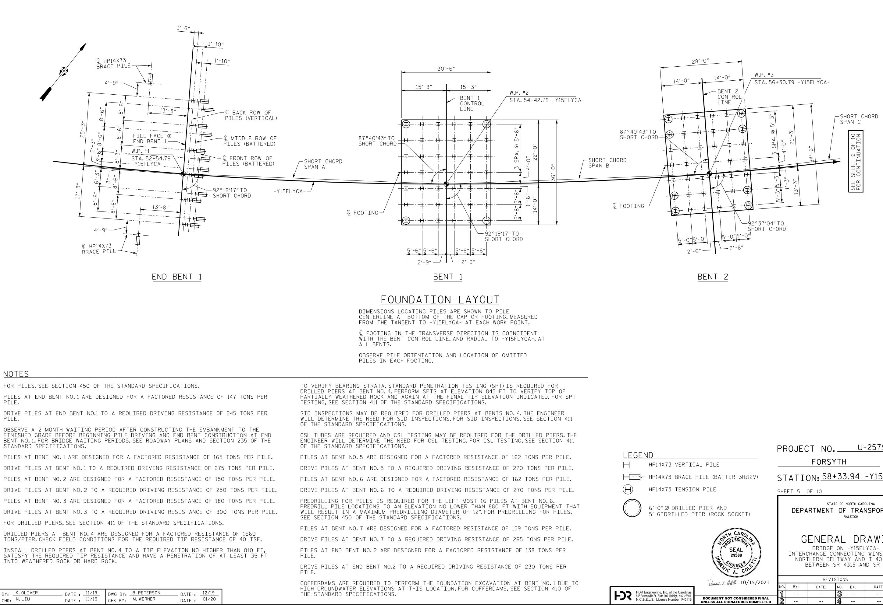
FOR DRILLED PIERS, SEE SECTION 411 OF THE STANDARD SPECIFICATIONS. DRILLED PIERS AT BENT NO.4 ARE DESIGNED FOR A FACTORED RESISTANCE OF 1660 TONS/PIER.CHECK FIELD CONDITIONS FOR THE REQUIRED TIP RESISTANCE OF 40 TSF.
