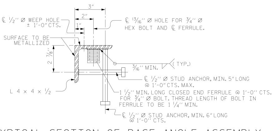
TYPICAL SECTION OF BASE ANGLE ASSEMBLY
