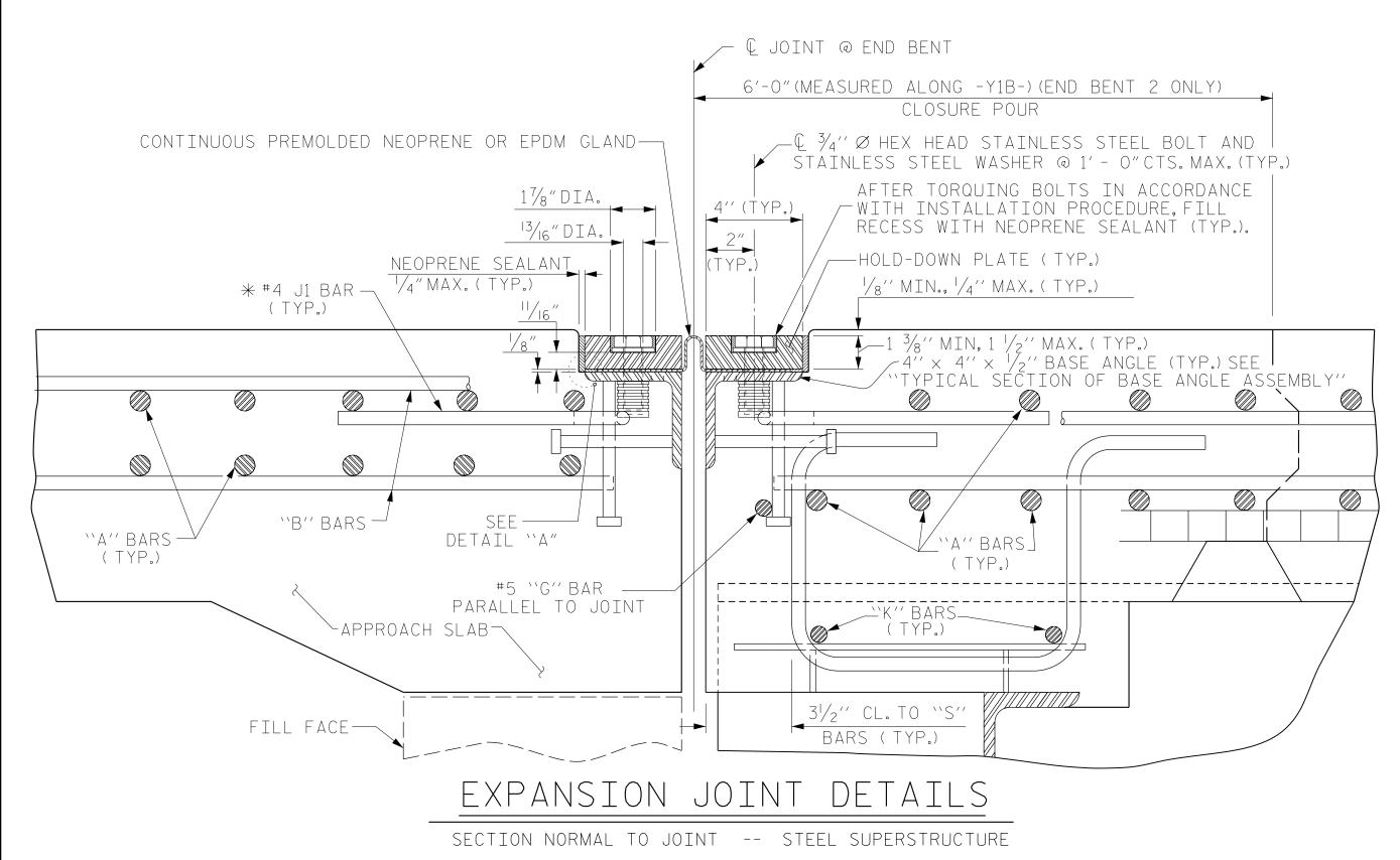
\* THE QUANTITY OF #4 J1 BARS ON THE BILL OF MATERIAL IS BASED ON 1'-O"CENTERS. J1 BARS SHALL BE PLACED AT EACH VERTICAL STUD ANCHOR BOLT. IN THE EVENT THAT THE NUMBER OF VERTICAL STUD ANCHORS EXCEEDS THE NUMBER OF J1 BARS SPECIFIED, ADDITIONAL J1 BARS WILL NOT BE REQUIRED.
