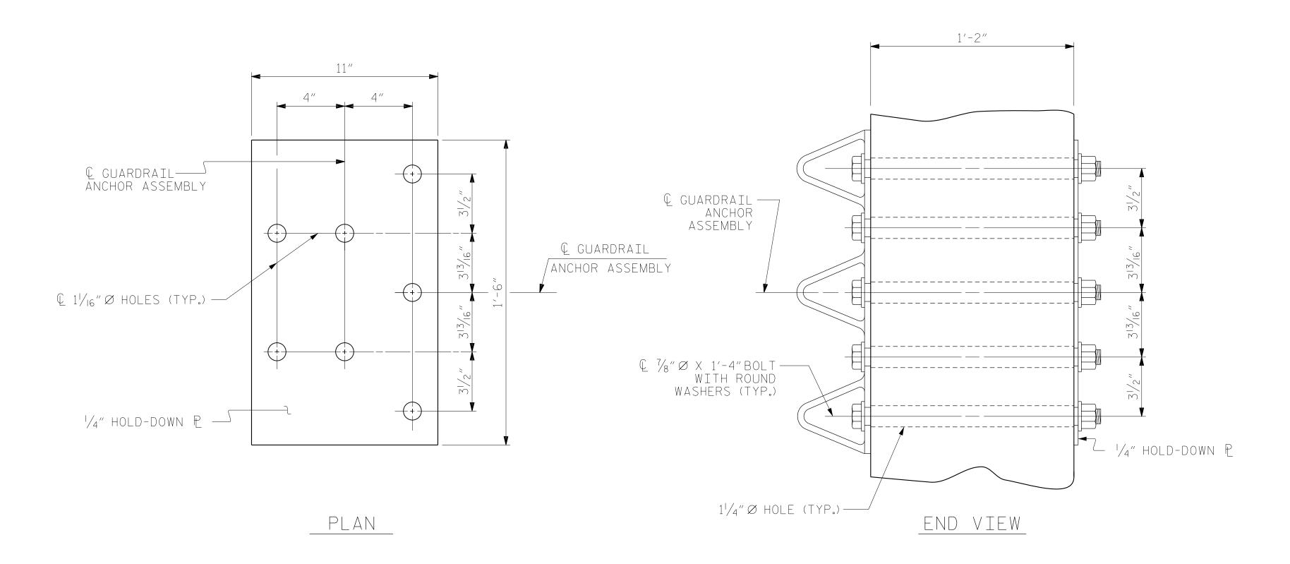
GUARDRAIL ANCHOR ASSEMBLY DETAILS
