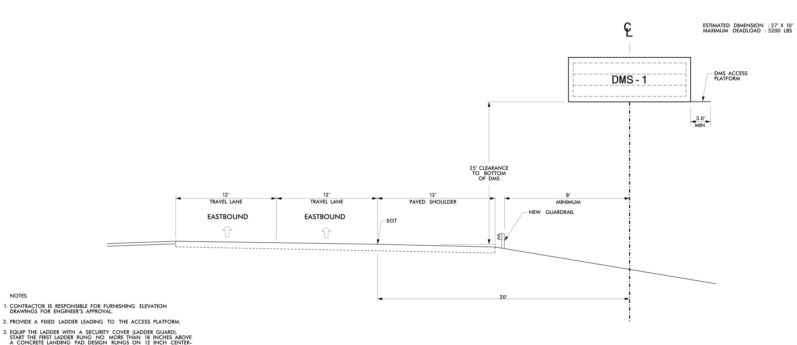
TO-CENTER TYPICAL SPACING. 4. INSTALL A CONCRETE LANDING PAD MEASURING A MINIMUM 4 INCHES DEEP, 24 INCHES WIDE, AND 36 INCHES LONG DIRECTLY
