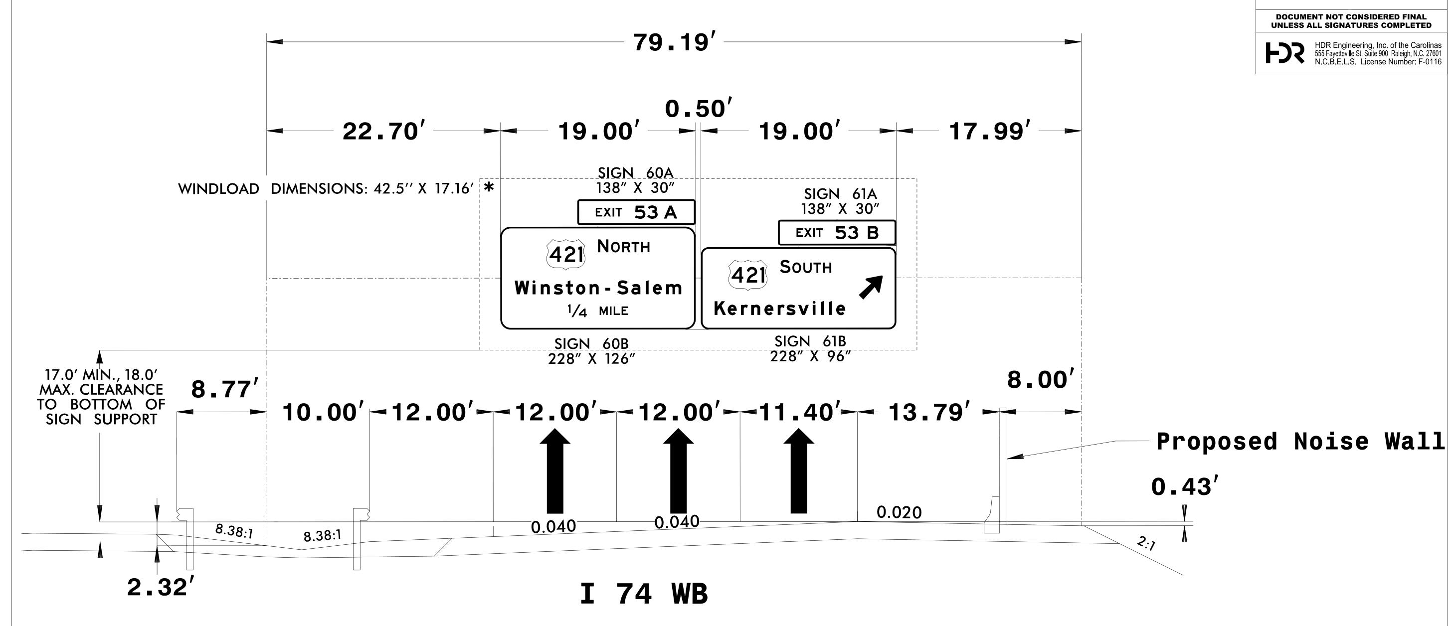
IF THE CONTRACTOR BIDS ALUMINUM SIGN STRUCTURE, EACH SHALL BE PROVIDED WITH AN APPROVED HIGHWAY TRUSS DAMPER DEVICE IN ACCORDANCE WITH AASHTO SPECIFICATIONS.
